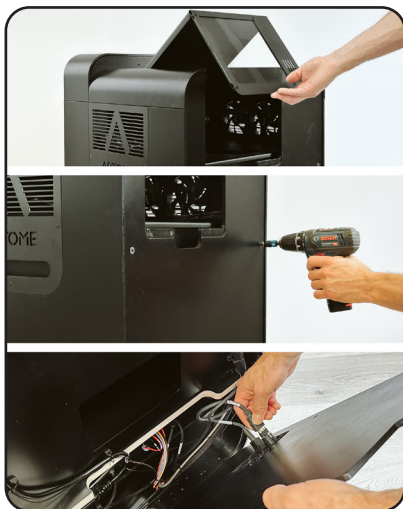
4. Open the lens latch. Remove the back cover (HEX4) and disconnect the pass-through cables
