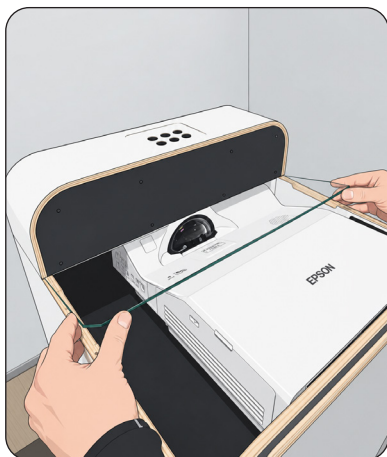
10. Reinstall the glass.
