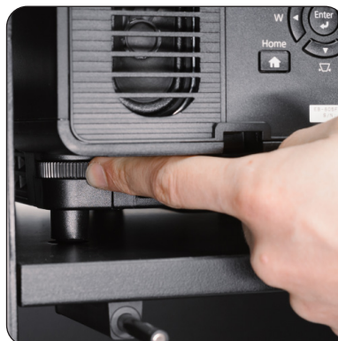
8. Lower the projector legs to alignment holes.
