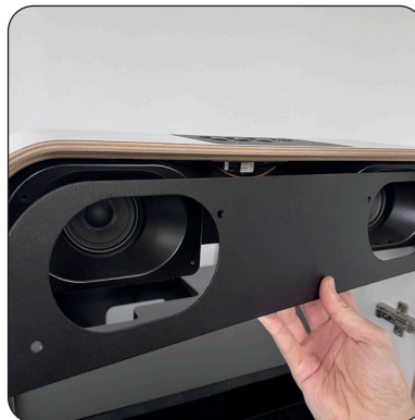
5. Remove the speaker panel cover with PH2 tool.
