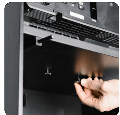
9. Fix the projector to cabinet with the provided thumb screws.
