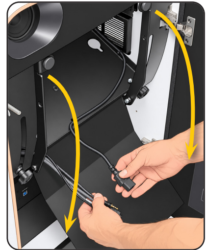
3. Open the front cover and place the cables on the cover plate.
