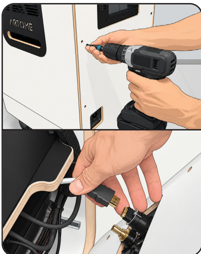
4. Remove the back cover (HEX3) and disconnect the pass-through cables.
